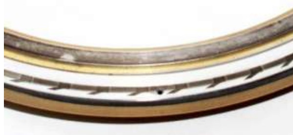
Figure 6. Sleeve of face seal with microgrooves
