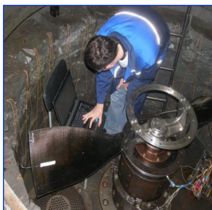
Figure 2. The carbonplastic fan blade installed on a spin rig.
