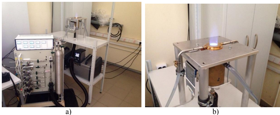
Figure 1 - Test rig to measure S_L : (a) general view, (b) burner device.
