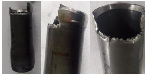
Figure 8. Cylinder spinning defects
