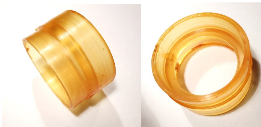
Figure 6. Bushings of worm wheel, free from defects - the correct parameters of the injection process
