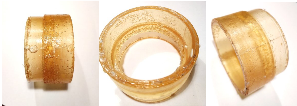
Figure 5. Worm wheel bushing: a) having defects on the outer and inner surface, b) having defects only on the inner surface
