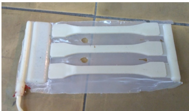
Figure 2. Molded samples (paddles) for tensile strength analysis made of PDCPD
