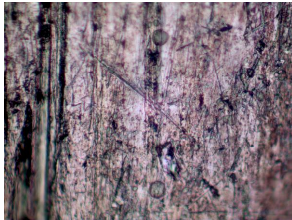
Figure 6. Welding zone of brass
