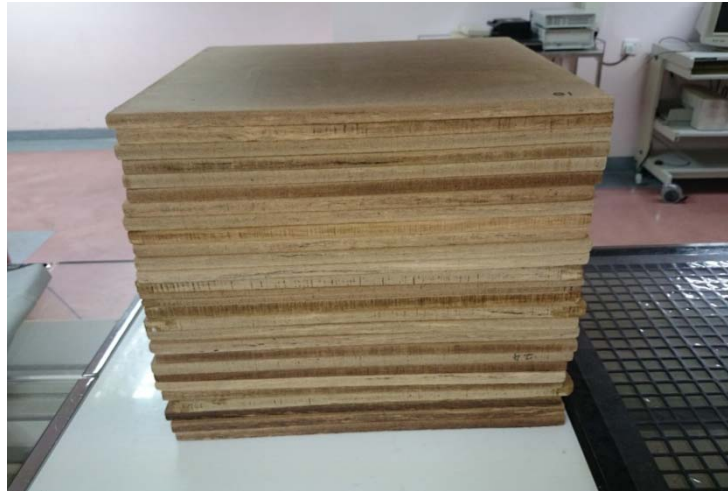
Figure 1. The fabricated Rhizophora spp. particleboard phantoms
