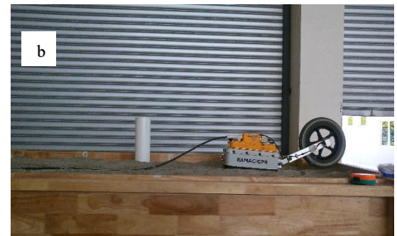
Figure 3. (a) Photograph of PVC pipe buried at the depth of 0.60 m, and the PVC pipe is in L-shape to inject water for water leaks simulation, (b) 800 MHz shielded antenna is perpendicular along the PVC pipe.
