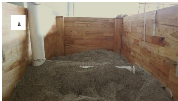
Figure 3. (a) Photograph of PVC pipe buried at the depth of 0.60 m, and the PVC pipe is in L-shape to inject water for water leaks simulation, (b) 800 MHz shielded antenna is perpendicular along the PVC pipe.
