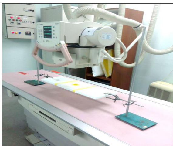
Figure 1. In air measurement setup.
