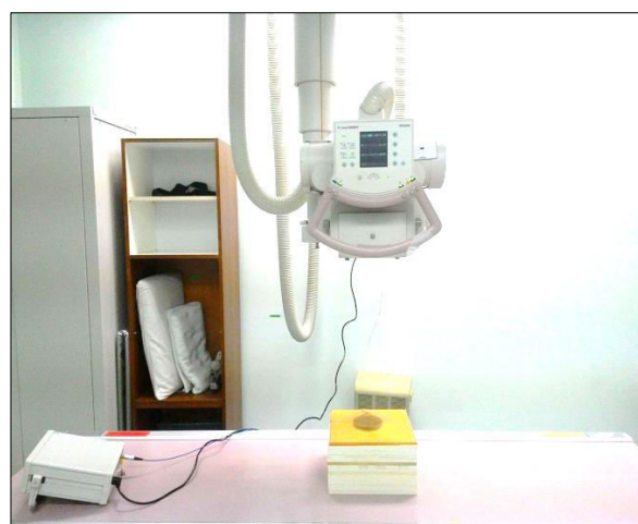
Figure 2. Phantom measurement setup.
