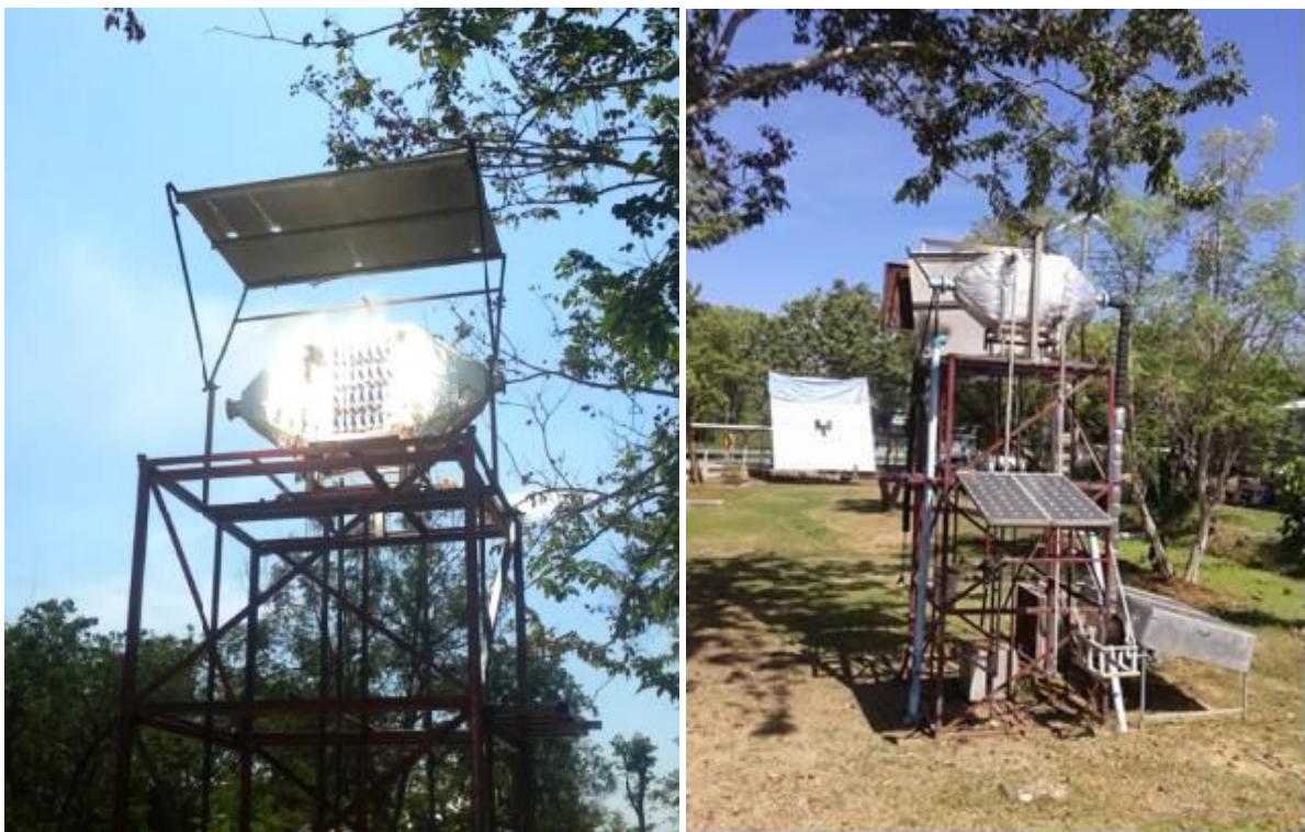
Figure 3. Photos of insulated solar tower receiver used in this study.
