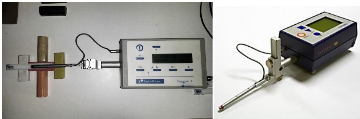
Figure 7. Measuring configuration for roughness measurement – roughness tester Surtronic 3+
