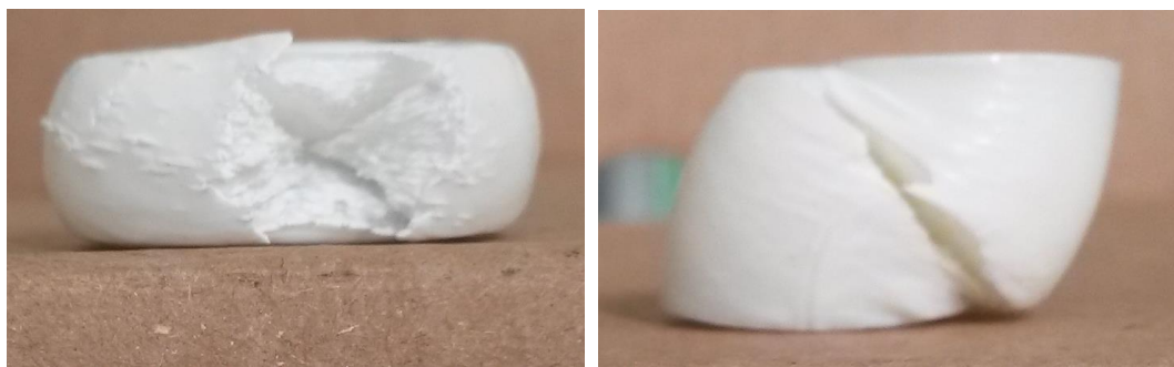
Figure 4. Two failure modes of deformation. Symmetrical deformation (left). Specimen collapsing to the side (right)
