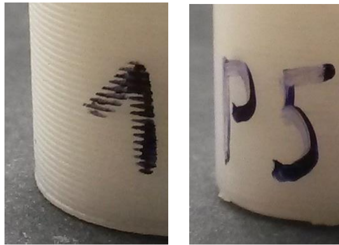
Figure 6. Presentation of different surface quality before (left) and after (right) vapor smoothing 5 min
