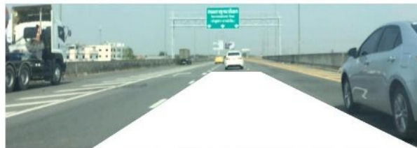
Figure 16. The mistake from the detection because of the heavy shadow.
