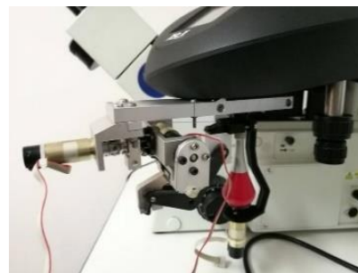
Figure 4. Slave arm is added on micromanipulator
