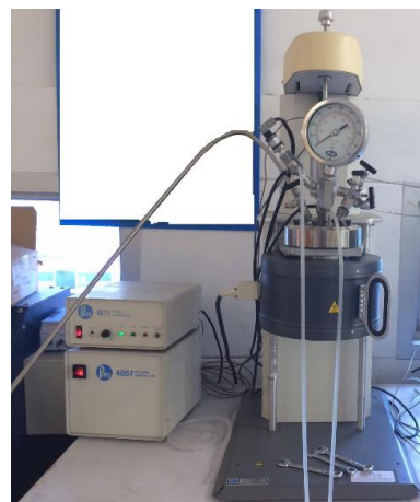
Figure 2. Parr reactor model 4857
