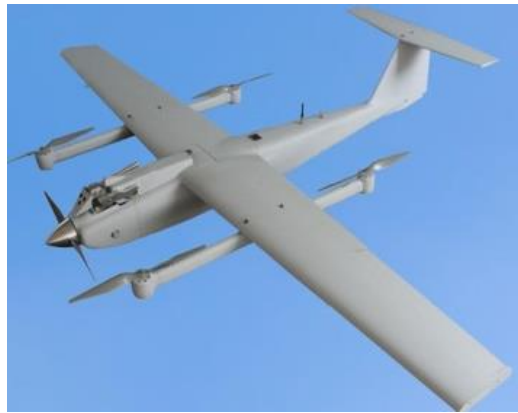
Figure 1: Hybrid Aircraft comprising a quad-copter, fixed wing and a forward thrust rotor
