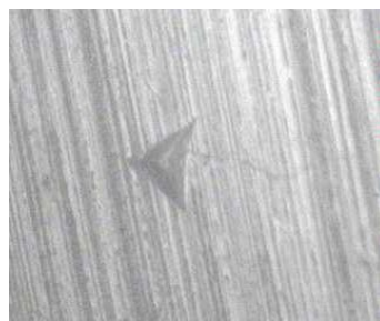
Figure 6. Indentation on dorsal cortex with micro-crack at peak load of 200 mN.
