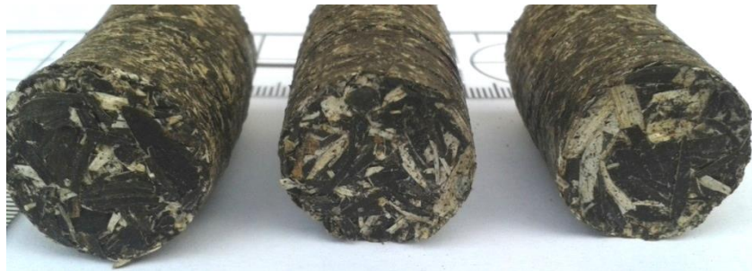
Figure 11. Binding of raw feedstock particles in sunflower hulls briquettes.
