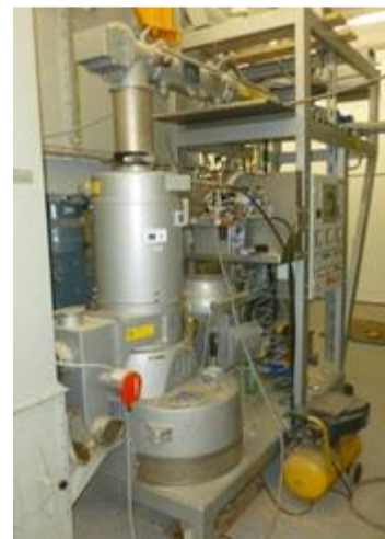
Figure 2. Pelletizing press KAHL 33-390.
