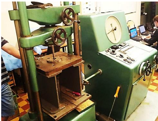
Figure 1. Hydraulic press with experimental pressing stand.
