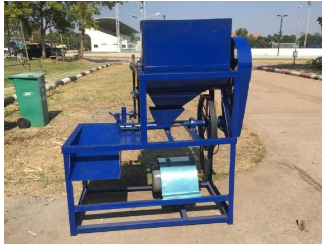
Figure 2. Charcoal briquette machine with a screw compressor.
