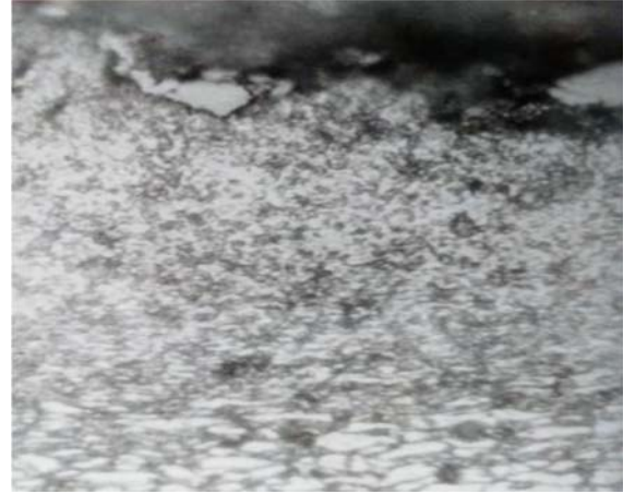
Figure 8. Optical micrograph of subsurface for the worn surface of AISI3315 steel (x200, Sliding direction is from left to right)
