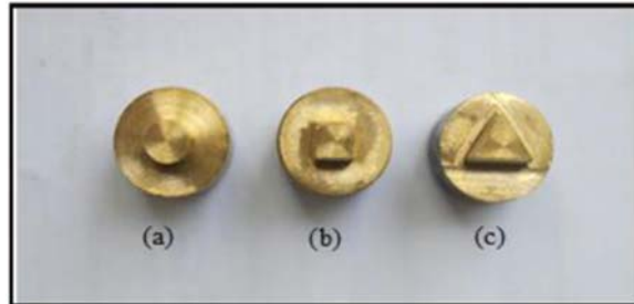
Figure 2. The utilized tips of indenter: (a) Circle; (b) Square; (c) Triangle.
