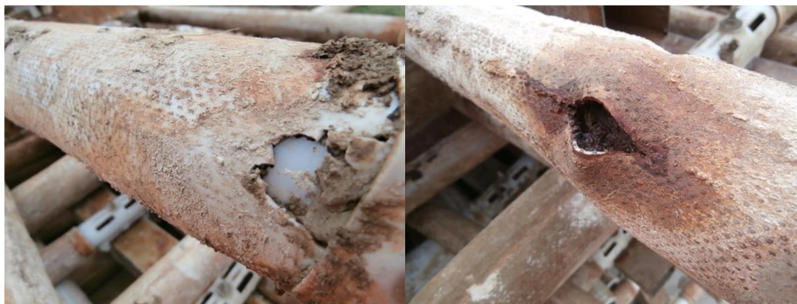
Figure 4. Corrosive effect of \text{FeCl}_3 about aeration system
