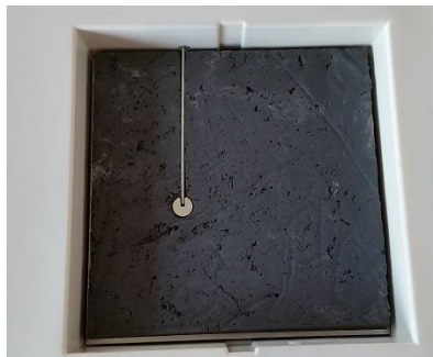
Figure 3. The way the thermocouples are mounted and the material sample are fitted inside the calorimetric chamber
