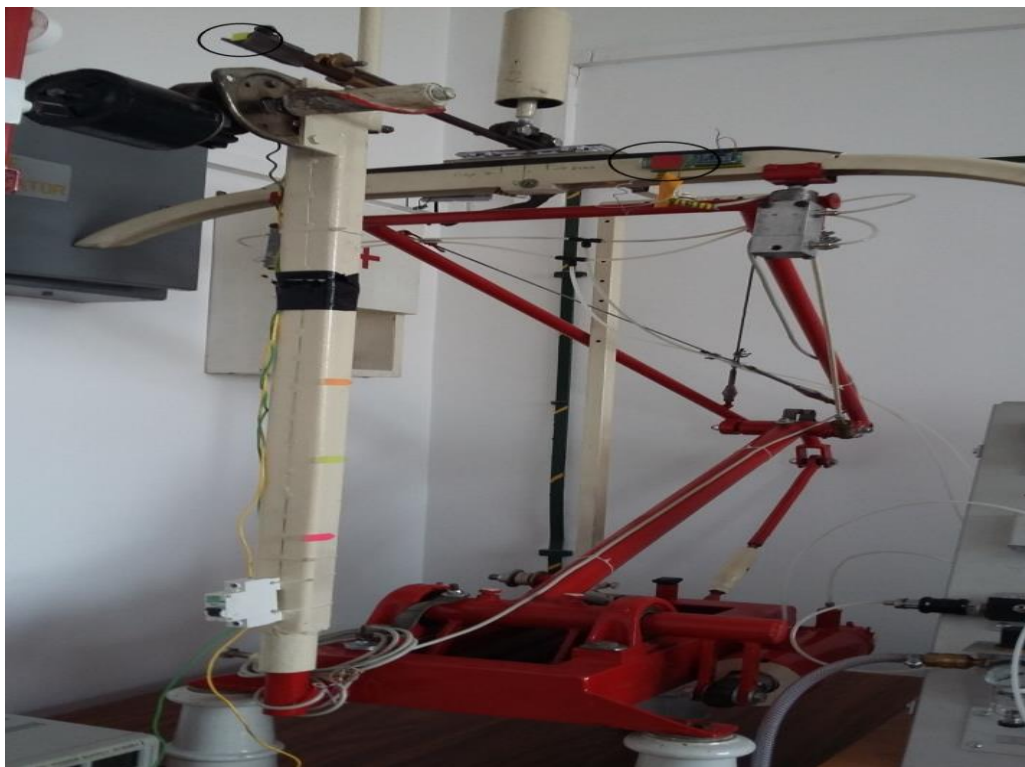
Figure 3. The laboratory model of the pantograph made at 1:2 scale
