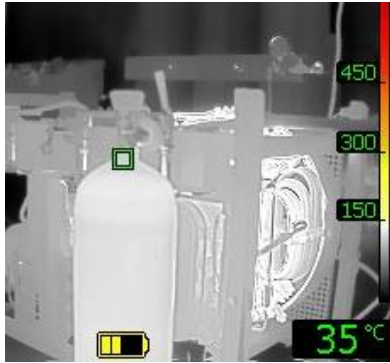
Figure 4. Temperature intensity at valve, comp. bottle
