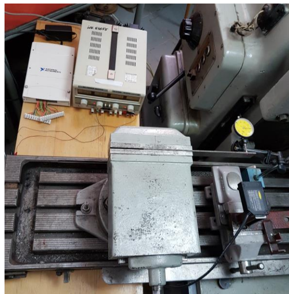
Figure 3. Setup for the sensor calibration made before employing it in the operation monitoring process
