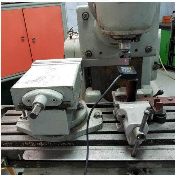
Figure 2. Experimental stand, consisting of a universal milling machine, machined piece and the optical sensor
