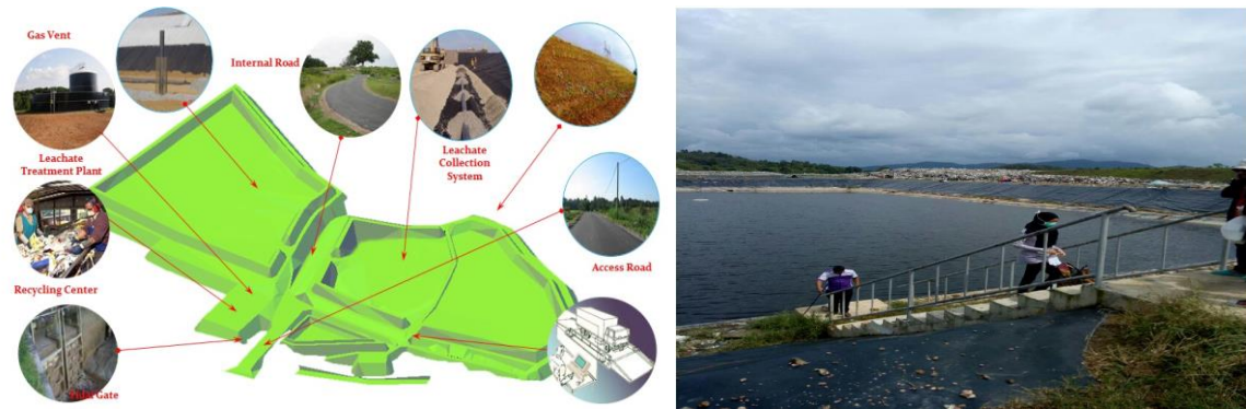
Figure 1. Sungai Ikan Landfill illustrated by Hexagon Energy with the Leachate Retention Ponds
