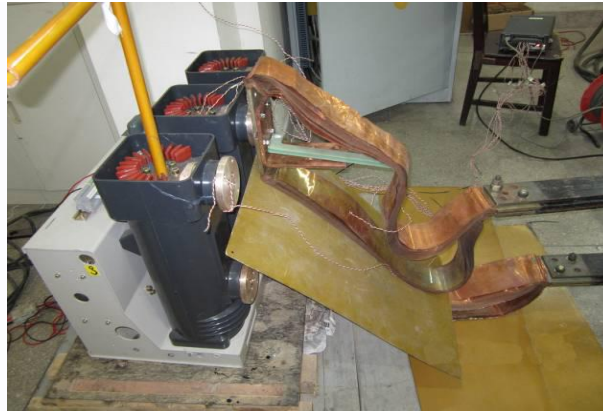
Figure 7. General circuit diagram when flexible coupling was added into terminal.
