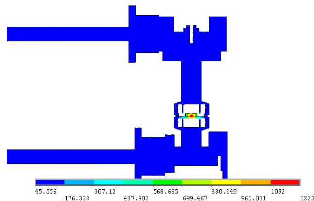
Figure 10. Transient temperature rise nephogram of the vacuum interrupter at the longitudinal profile.
