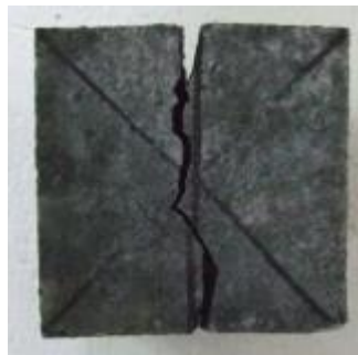
Figure 4. Fracture form of dumbbell type specimen.
