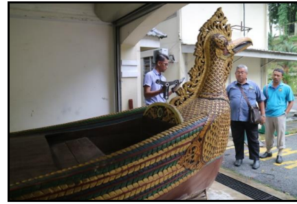
Figure 5. Scanning process of Freestyle3D. Figure 6. Scanning process Freestyle3D.
