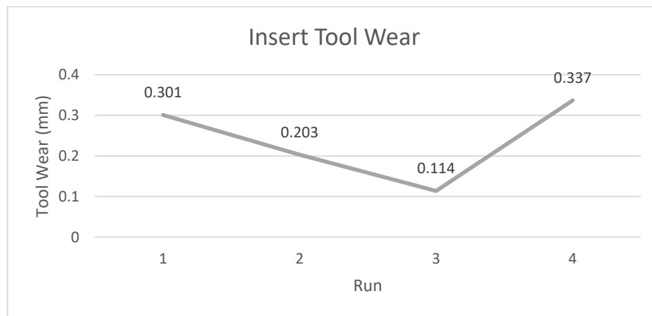
Figure 4. Insert tool wear on the preliminary test of AISI H13 milling
