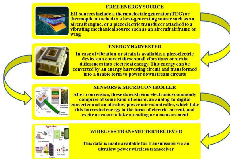
Figure 1. Schematic of general mechanism of energy harvesting principle.
