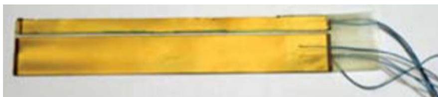
Figure 4. Schematic of the multilayer composition of the piezoelectric flag [15].
