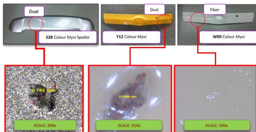
Figure 2. Sample contamination of dust and fibre in painting line (Source from Combat Coating (M) Sdn Bhd ).
