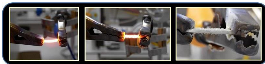
Figure 1. Electric current heating applied into ceramic bar for ZnO crystal growth. It is shown on the 3 rd figure the crystal grew on the surface of ceramic bar.
