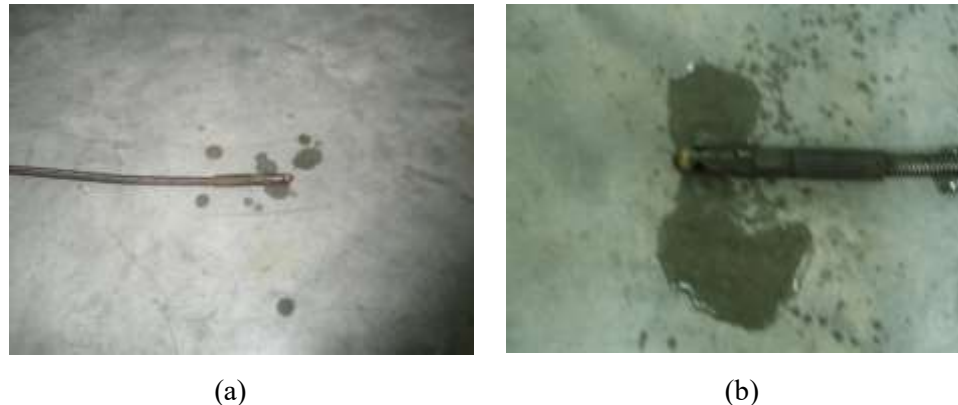
Figure 9. The gas probe in modified muffler expels lots of water vapor: (a) without a catalytic converter, (b) with the chrome-coated copper metallic catalytic converter.
