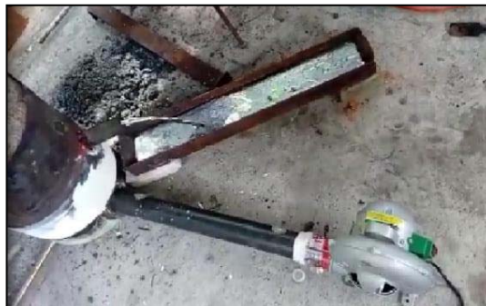
Figure 6. Traditional oxygen bottom blowing process
