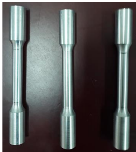
Figure 3. Specimen for tensile testing
