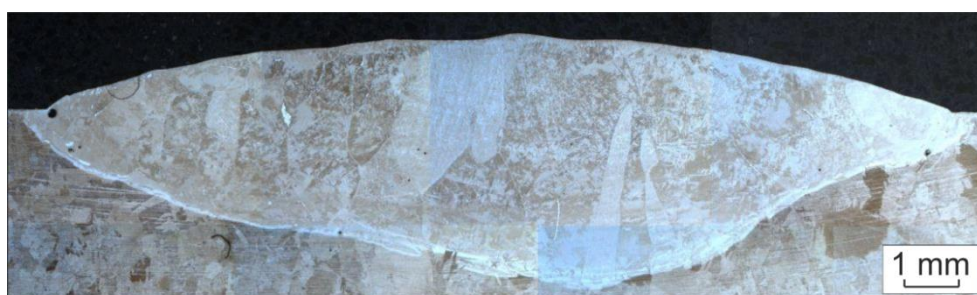
Figure 1. The cross-section of the Ti-Nb layer cladded by an electron beam in a protective media of argon.
