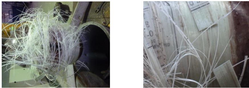
Figure 3. The shape of the burst composite cylinder
