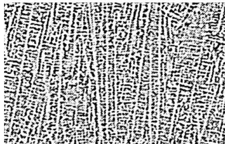
Figure 3. Micrograph of columnar crystal of the secondary cooling zone in transverse section of 380 mm x 280 mm rectangular bloom of steel 20.
