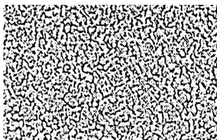
Figure 4. Equiaxed grain band: horizontal area of 300mm×1650 mm blank from medium carbon steel (0.23% W(C)).
