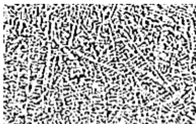
Figure 9. Micrograph of the secondary dendrite in the transverse section of medium carbon steel (0.16%W(C)) in 230mm×1650mm blank.
