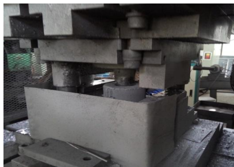
Figure 4. A hydraulic press with a die.
