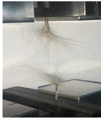
Figure 3. A photo of the moment of the crack of the basalt roving
