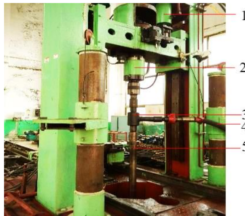
Figure 7. Simulation test device for the horizontal well jarring tool string.
