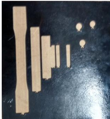
Figure 1. Goat hair epoxy composite
