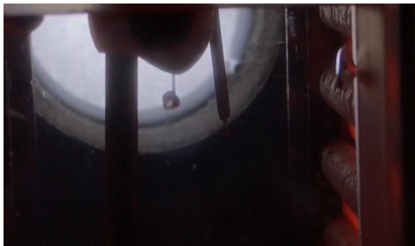
Figure 2 Ethanol gel droplet inside of the combustion chamber with electric furnace
