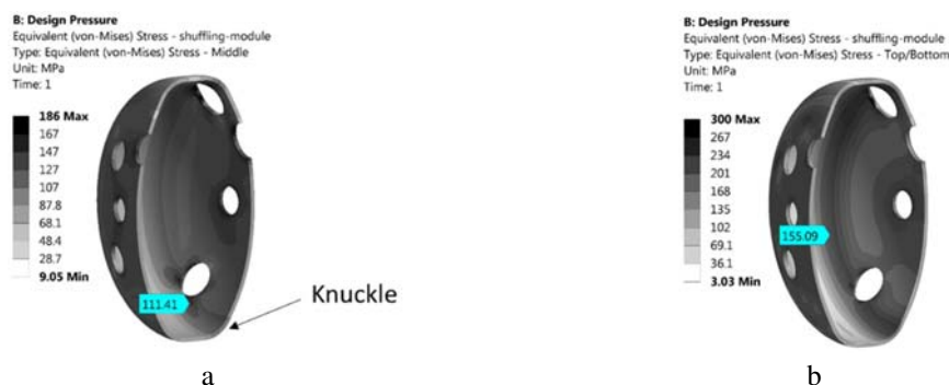
Figure 8. Membrane stress (a) and membrane plus bending stress (b) in the shuffling module.
