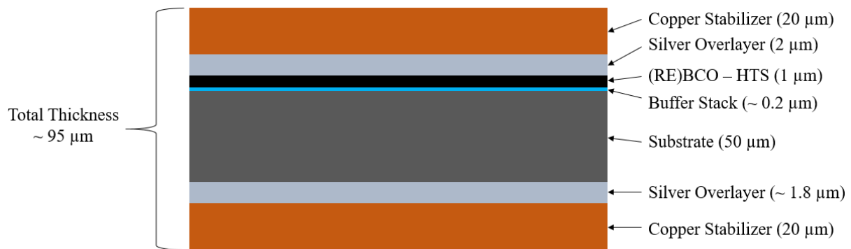
Figure 2. Materials and layer thicknesses of SuperPower SCS4050 HTS tape (not to scale) [3].
