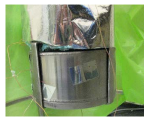
Figure 10. HTS test configuration: Aluminum 6061 plate showing the placement of the HTS material (left) and attachment of HTS and aluminum plate assembly to the bottom of the cold mass (right).
