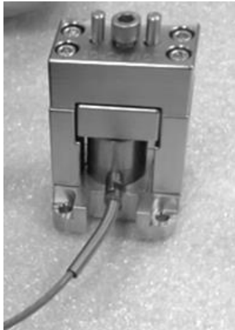
Figure 2. Force test load cell installation.
