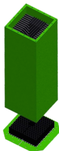
Figure 1. Simulation environment: This thick walled rectangular aluminum box with black-painted honeycomb epoxied to the insides provides an environment with an emissivity close to 1.0.
