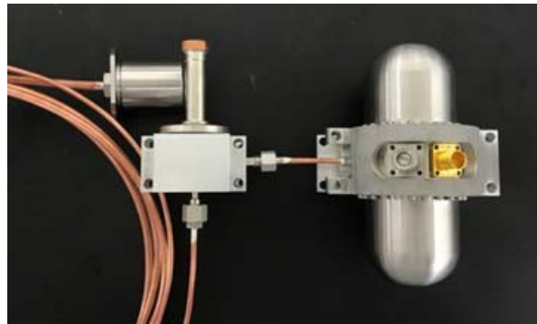
Figure 4. The 800 g micro coaxial SPTC operating at 144 Hz.
